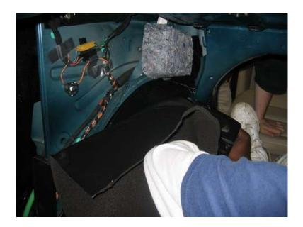
Lay the single sheet of HushMat Silencer Megabond over the wheel well with the white release paper intact. Measure and cut with scissors or utility knife. Peel back one straight edge of the white release paper and adhere the Silencer Megabond directly on top of the HushMat Ultra on the Wheel Well. Repeat this step for both wheel wells.
