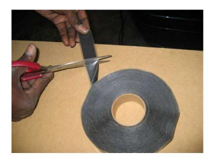
An important step is to secure all wires and cables in the trunk using HushMat Quiet Tape. Cut the Quiet Tape in 3-4 inch strips.
