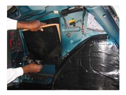
Treatment of the rear quarter panels is required due to the thin gauge sheet metal and the small amount of interface with the vehicle frame. These expansive panels are loosely supported and resonate. Cut the large sheet of HushMat Ultra in half and press it onto the inside of the outer quarter panel skin through the frame.
